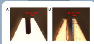
Figure 3. Closed back side (A) and open front side (B) of y-junction pin makes a 3-sided channel at the tip only. This is due to incomplete DRIE etch at the thinnest part of the channel which is the tip. Remaining parts of channels are 2-sided.
