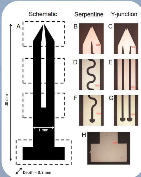
Figure 2. Schematic (A) of pin design and pictures of back side of tip (B, C), channel (D, E), top of channel (F, G) of serpentine and y-junction two-pronged blunt pin designs, respectively. Pins are attached to the wafer (H) by the side. Top of channels feature a stop valve [2] which allows accurate liquid metering by stopping liquid at the top of the microchannel. Scale bars in B through H are 200 microns.
