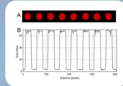
Figure 4. Spot intensity profile printed with y-junction pin. Analyzed using ImageJ.
