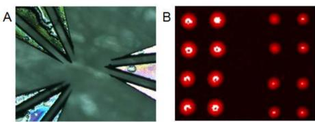
Figure 1. Tips of three-pronged Si quill pins with double channel (A) and printed fluorescent spots (B) from four pins (four groups of four) printed simultaneously on a nitrocellulose slide. Tips of the three-pronged pins are sensitive to variation in the microfabrication processes which lead to different spot sizes by different pins.
