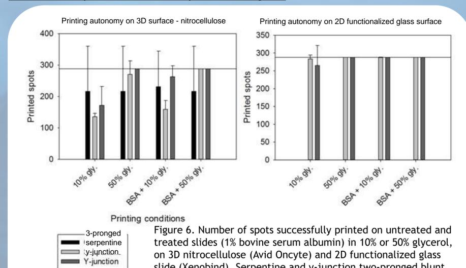
Figure 6. Number of spots successfully printed on untreated and treated slides (1% bovine serum albumin) in 10% or 50% glycerol, on 3D nitrocellulose (Avid Oncyte) and 2D functionalized glass slide (Xenobind). Serpentine and y-junction two-pronged blunt pins print for the full run (reference line, 288 spots) while the three-pronged pins are emptied before printing run is finished.
