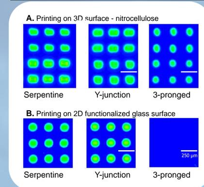
Figure 5. Spot morphology printed on 3D nitrocellulose (A) and 2D functionalized glass surface (B) shows that the 2-pronged serpentine and y-junction pins successfully print on all surfaces including glass. Scale bars are 250 microns.
